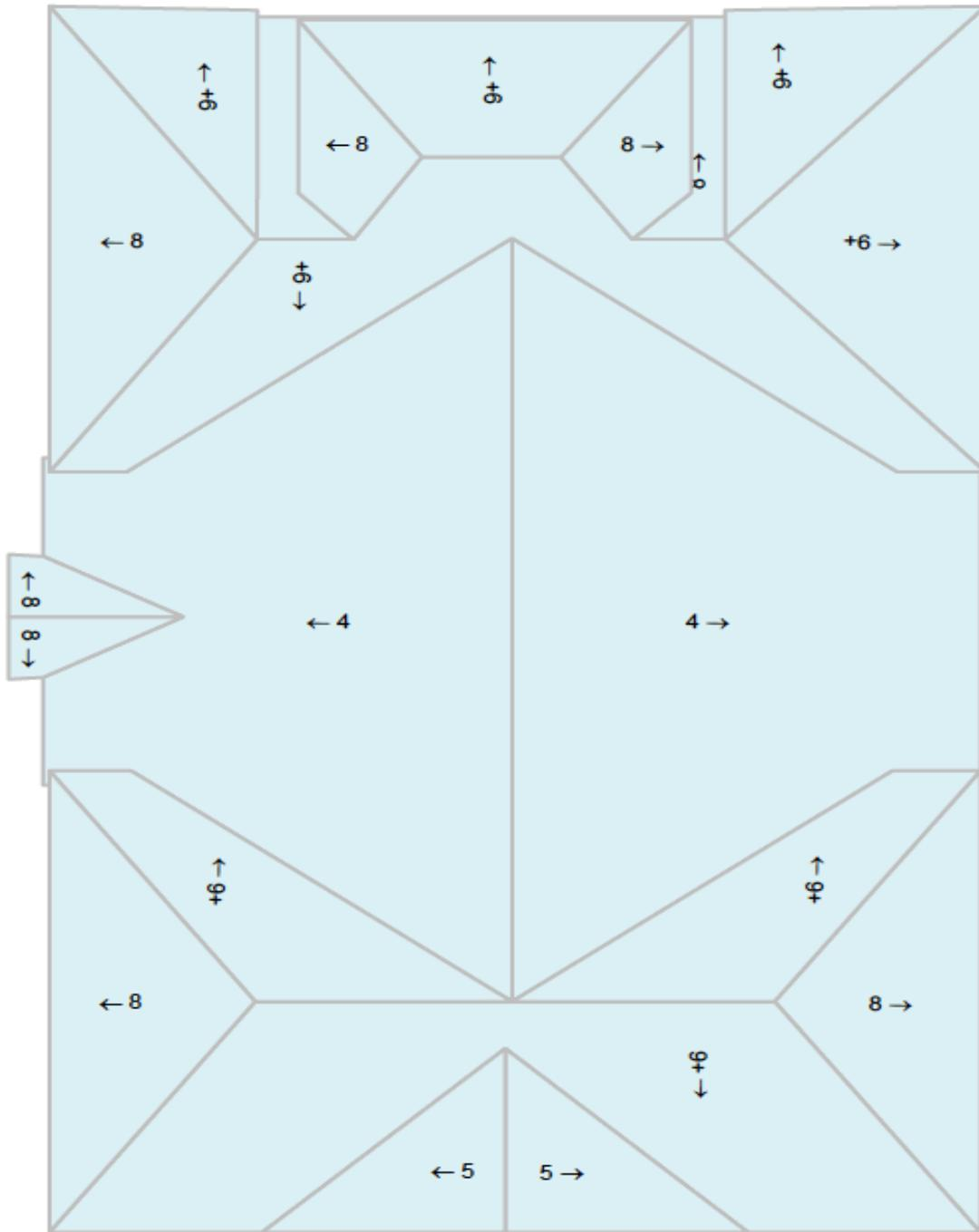
Figure 4: Pitch values are shown in inches per foot, and arrows indicate slope direction. (To be confirmed by Bidders.)
